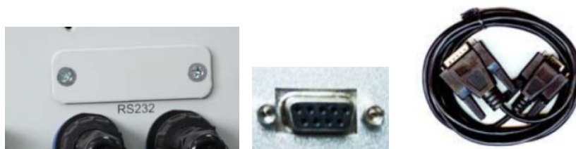
Fig. 10 RS232 serial port and special RS232 cable
