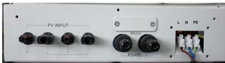
Fig. 7 Connections available on inverter bottom and relevant marking
